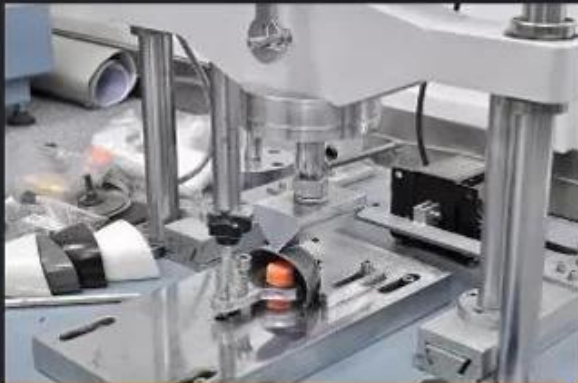
Toecap Test \geq 200 Joules
