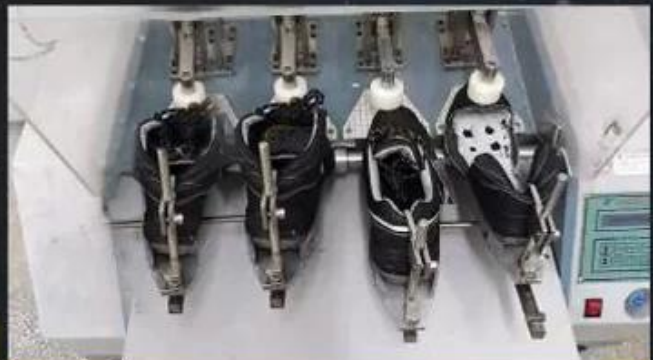
Flex Tester \geq 36,000 T
