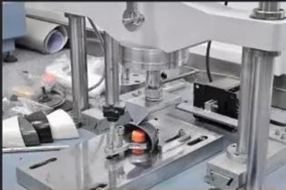
Toecap Test \geq 200 Joules
