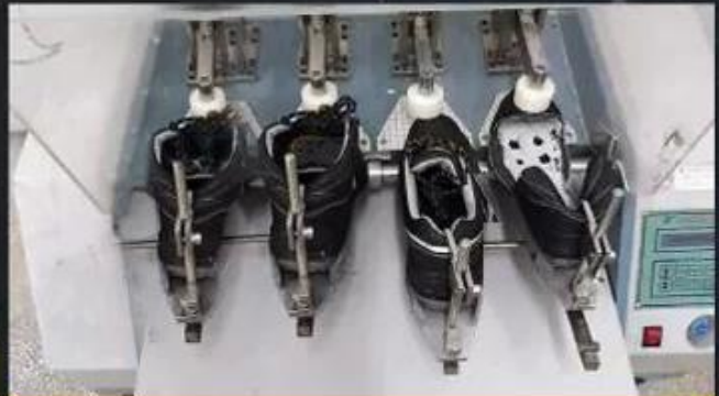
Flex Tester \geq 36,000 T
