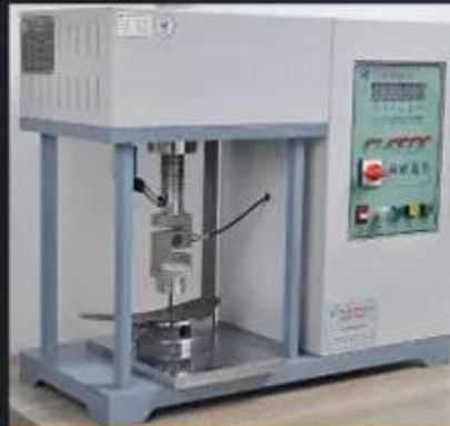
Midsole Test \geq 1200 Newtons
