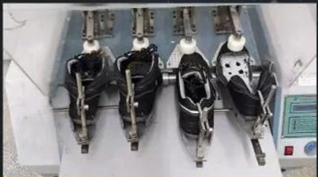
Flex Tester \geq 36,000 T
