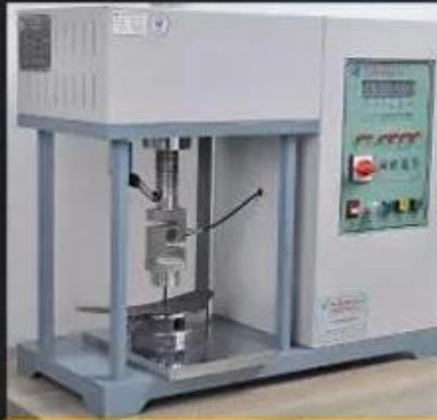
Midsole Test \geq 1200 Newtons
