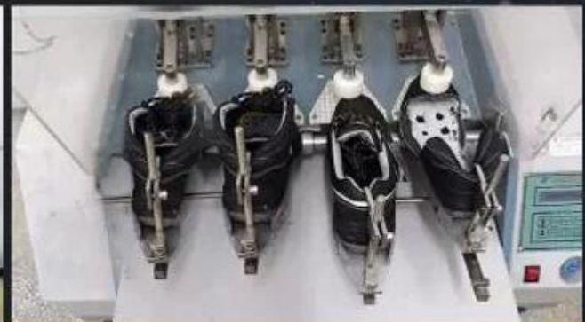
Flex Tester \geq 36,000 T
