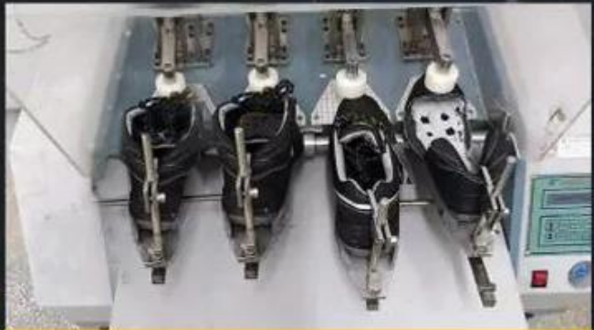
Flex Tester \geq 36,000 T
