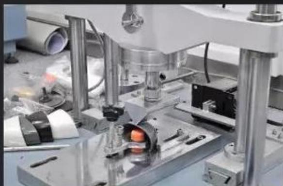
**Toecap Test  $\geq 200$  Joules**
