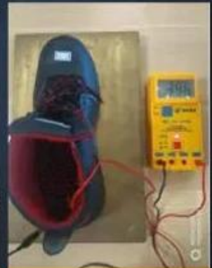
ESD Anti-Static Test
