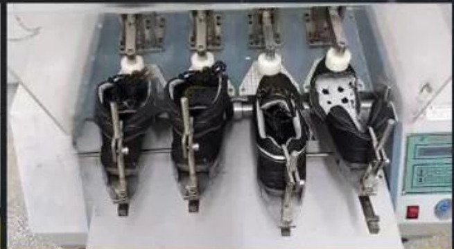
Flex Tester \geq 36,000T
