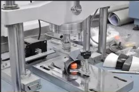
Toecap Test \geq 200 Joules
