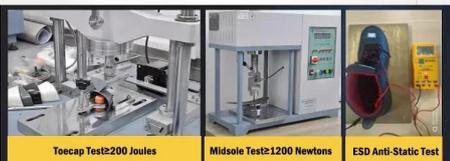
Toecap Test  $\geq 200$  Joules
