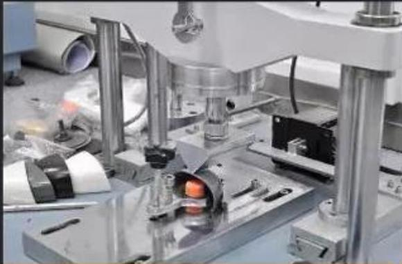
**Toecap Test  $\geq 200$  Joules**
