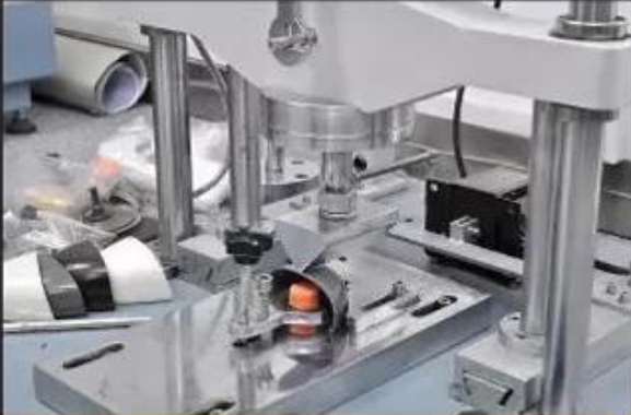
Toecap Test \geq 200 Joules
