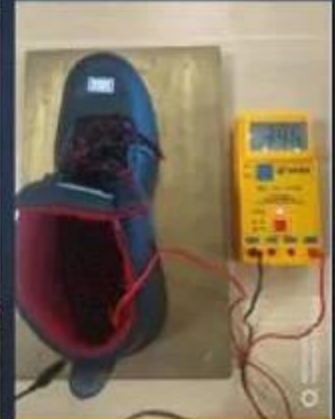
ESD Anti-Static Test
