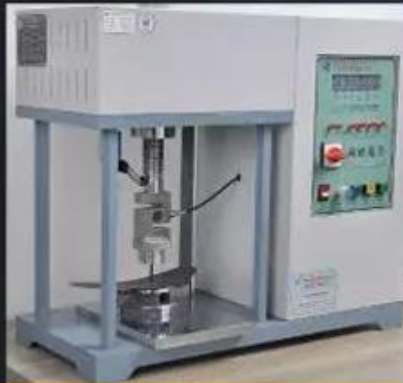
Midsole Test \geq 1200 Newtons
