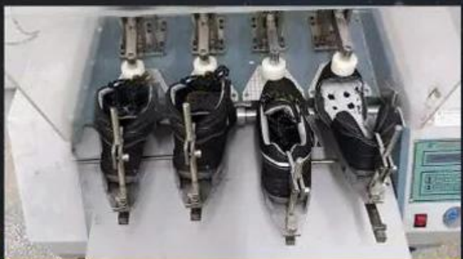
Flex Tester \geq 36,000 T
