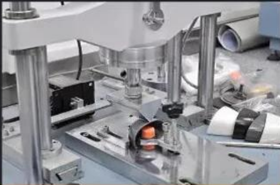
Toe cap Test \geq 200 Joules
