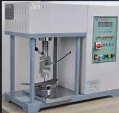
Midsole Test \geq 1200 Newtons
