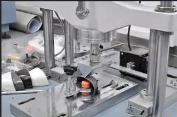
Toecap Test \geq 200 Joules
