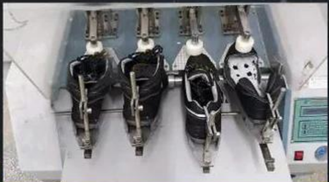
Flex Tester \geq 36,000 T
