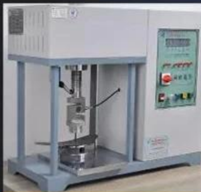
Midsole Test \geq 1200 Newtons
