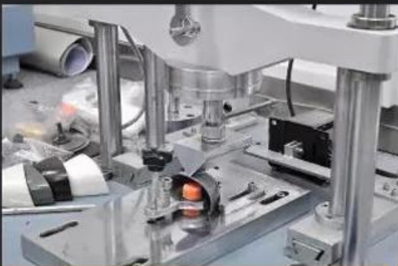
Toecap Test \geq 200 Joules
