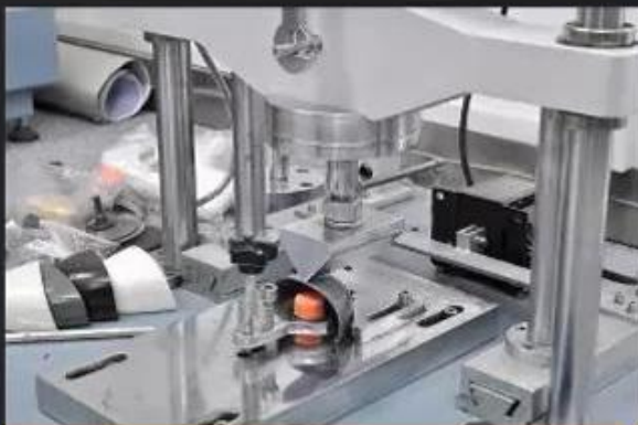
Toecap Test \geq 200 Joules
