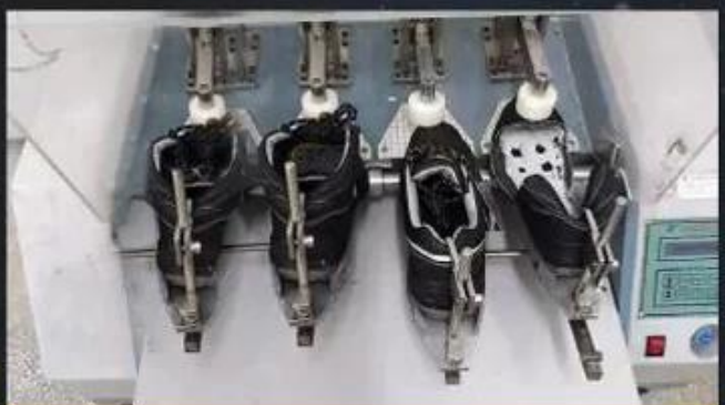
Flex Tester \geq 36,000 T
