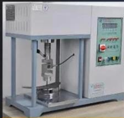
Midsole Test \geq 1200 Newtons
