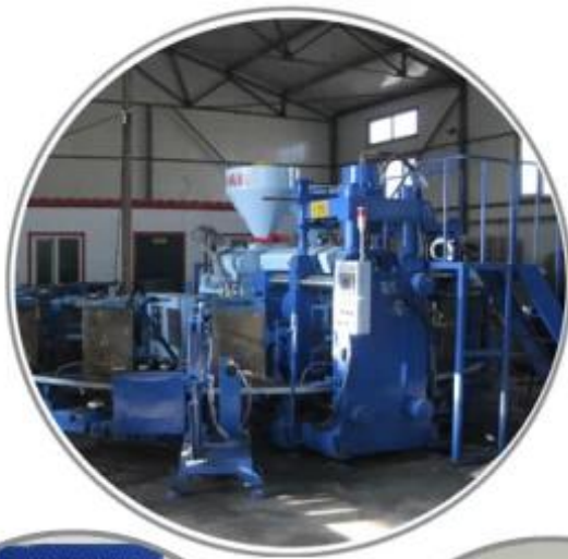
Automatic Injection Molding Machine
