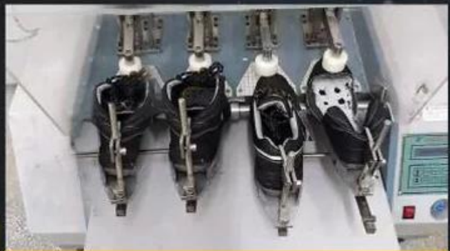
Flex Tester \geq 36,000 T
