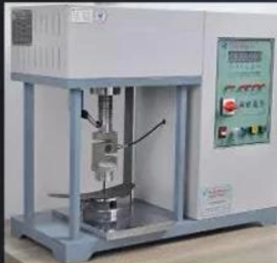
Midsole Test \geq 1200 Newtons
