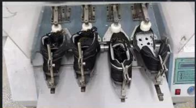
Flex Tester \geq 36,000 T
