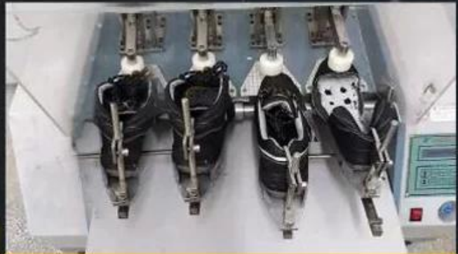
Flex Tester \geq 36,000 T
