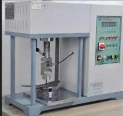
Midsole Test \geq 1200 Newtons
