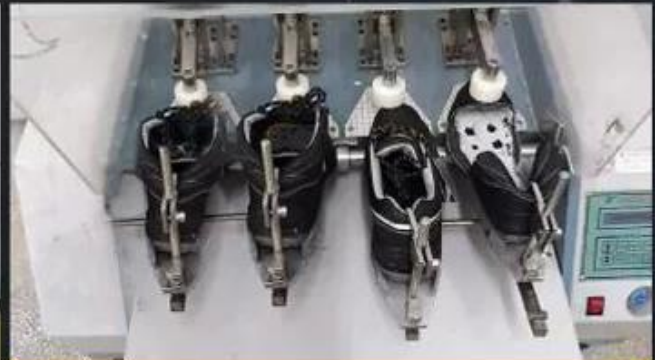
Flex Tester \geq 36,000 T
