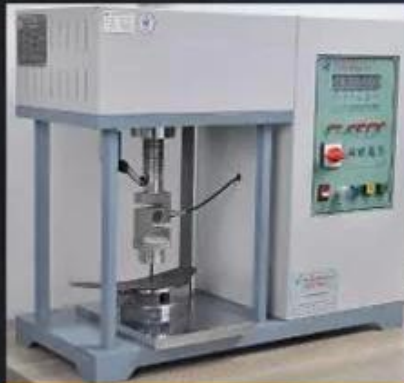
Midsole Test \geq 1200 Newtons
